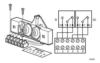
Fig. 1. Auxiliary switch parts and wiring.
